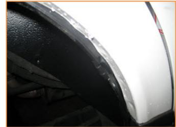
Press the Mudguard firmly on the surface on the rim, the car tape needs some pressure to reach its maximum strength.
